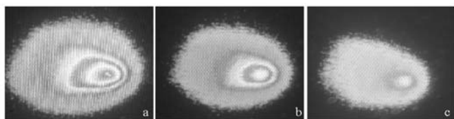
Fig. 3. Spatial distribution of the QC laser intensity, recorded with a thermal camera, for an incident power of (a) 47 mW, (b) 32 mW, (c) 15 mW. The orientation of the laser plane is vertical.
